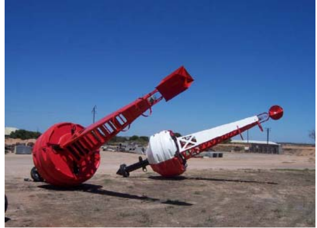
1770kg, 4 metre focal height. 2.4 metre diameter. Overall height 8.9 metres
